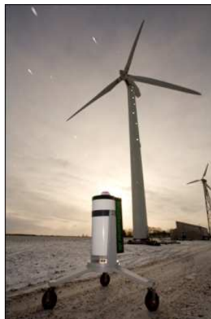
Figure 2b: A Short-Range WindScanner (R2D1) during field test at Risø DTU
