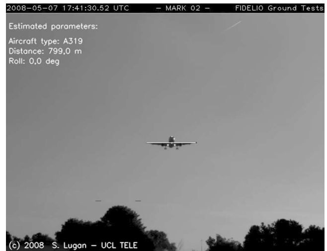
Fig. 14. Aircraft tracking video for distance computations for the wind data (refer to Fig. 15).
